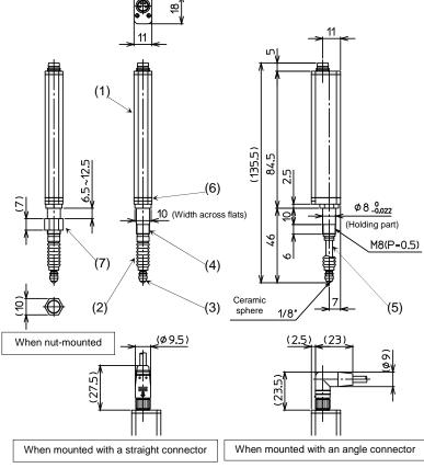
When connecting the connector, engage it firmly and tighten the threaded part securely. (Recommended tightening torque: 0.2 to 0.3 N·m)
